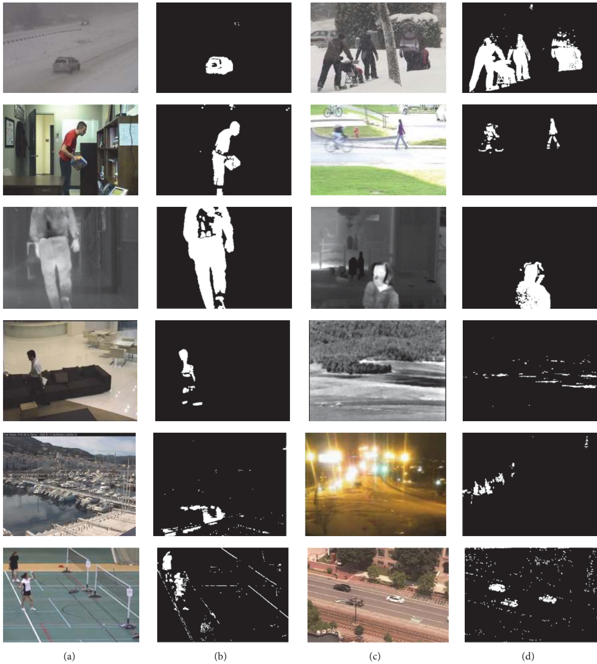
FIGURE 8: Detection results of other categories. (a) and (c): input test video; (b) and (d): detection results. The first row is the “Bad Weather” category, the second row is the “Baseline” category, the third row is the “Thermal” category, the fourth row is “Intermittent Object Motion” category and “Turbulence” category, the fifth row is “Low Framerate” category and “Night Videos” category, and the sixth row is “Camera Jitter” category and “PTZ” category.
