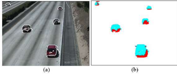
Fig. 12. Results on sequence Highway II. Note the similarity in the appearance of shadows and dark vehicles.
