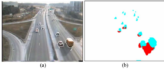
Fig. 12. Results on sequence Highway II. Note the similarity in the appearance of shadows and dark vehicles.
