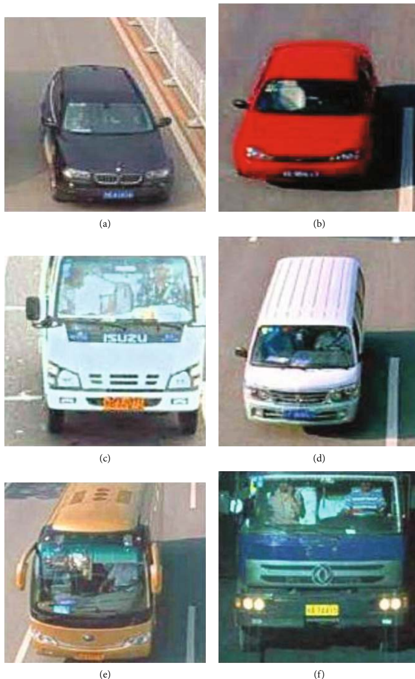
FIGURE 2: Sample images of BIT Vehicle Dataset: (a) SUV, (b) sedan, (c) minivan, (d) microbus, (e) bus, and (f) truck.
