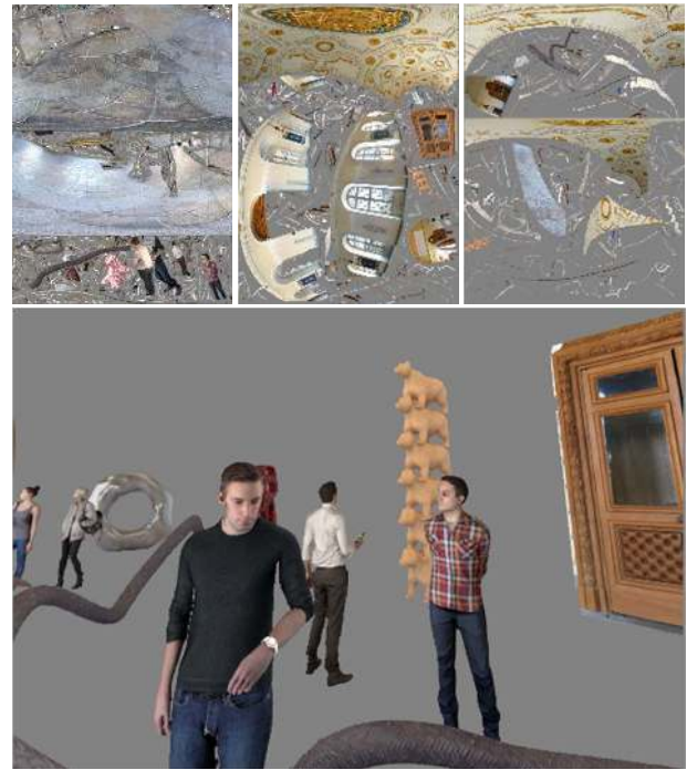
Fig. 9. Entity-based TMIV coding of Museum showing three atlases (out of four) in the top row, coding all entities. Rendering results of selected entities (representing foreground entities) in the bottom row.
