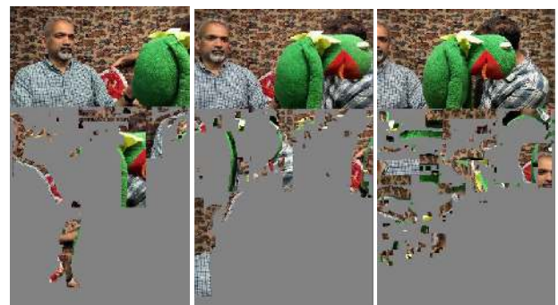
Fig. 8. Group-based encoding results using three groups (ordered left to right) for the Frog content. Each group has one atlas, each with one whole basic view (on the top) plus patches of multiple additional views.
