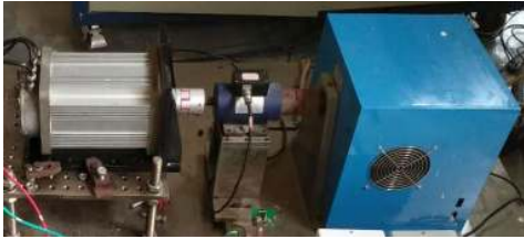
Fig. 7 Experimental setup for high speed PMSM
