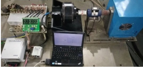
Fig. 6 Experimental setup for in-wheel motor
