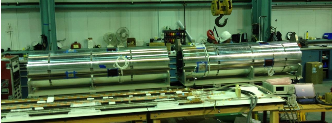
Fig. 6.7. Two half-length yoke-shell subassemblies, ready to be joined.
