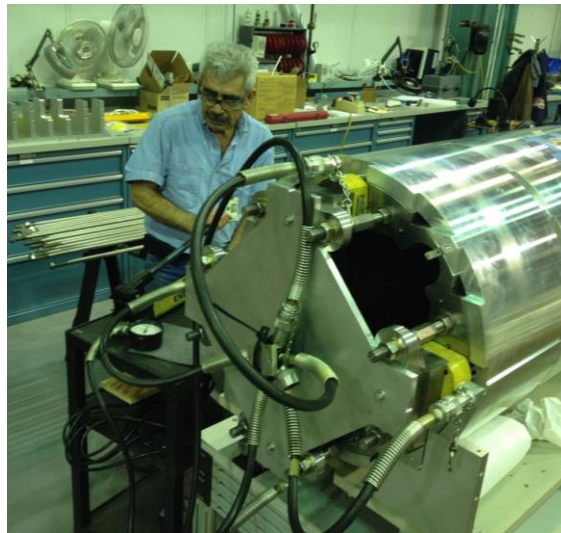
Fig. 6.8. Hydraulic rig for pre-tensioning the yoke tie rods.
