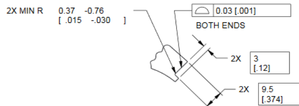
3.12: Yoke 3mm x 9.5mm gap key grooves.
