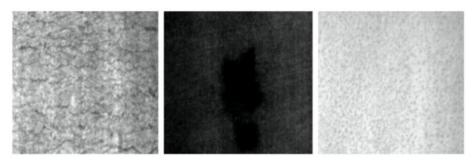
Figure 7. Defect images of crazing, patches, and pitted surface.
