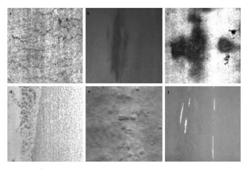
Figure 1. Different types of steel surface defects. (a) Crazing, (b) inclusion, (c) patches, (d) pitted surface, (e) rolled-in scale, (f) scratches.
