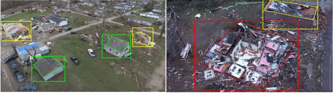
Figure 2. Visualization of our ISBDA dataset. The green, yellow and red polygons denote damages in Slight, Severe and Debris levels, respectively. The rectangles composed of solid lines represent damaged building bounding boxes. The polygons with dotted lines represent segmentation masks of damaged parts.
