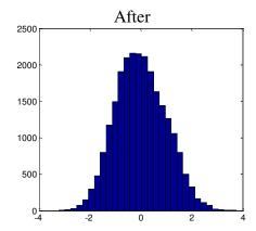
Unlike with the global CMVN, for this sample feature stream the overall shape of the feature stream distribution is approximately mapped to a standard normal distribution.
