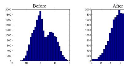
Notice that the overall distribution of the feature stream is warped to the standard normal distribution.
