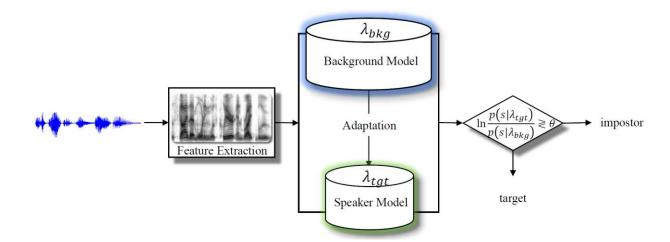
A speaker recognition system includes two primary components: a front-end and a back-end. The front-end transforms acoustic waveforms into more compact and less redundant representations called acoustic features. Cepstral features are most often used for speaker recognition. It is practical
