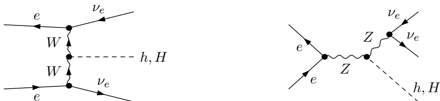
Figure 4.5: The tree-level diagrams for the process e^+e^- \rightarrow \bar{\nu}_e\nu_e \{h, H\} , consisting of the WW -fusion contribution (left) and the Higgs-strahlung contribution (right).
