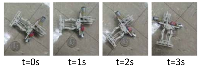
Fig. 18. Steering experimental result. Four individual frames extracted from a steering video.
