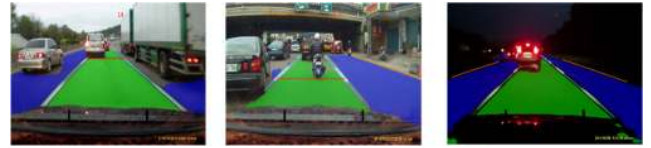
FIGURE 19. Qualitative results of forward collision warning system.
