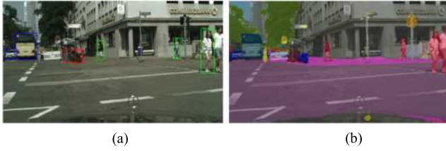
FIGURE 8. Illustration of common multi-task network output. (a) Detection prediction, (b) Segmentation prediction.
