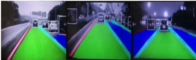
FIGURE 22. Qualitative results of object detection and segmentation predictions on TDA2x.
