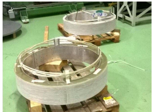
Fig. 6. The two coils of the prototype module after impregnation and machining of the external surface.
