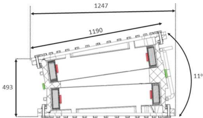
Fig. 9. Cross section of the TS prototype module highlighting the location of the spot heaters (red) on the coils and (green) on the housing shell. Dimensions are in millimeters.
