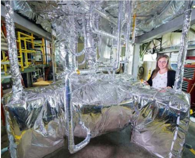
Fig. 5. Prototype with its custom thermal shield finalized and ready to be cold tested.
