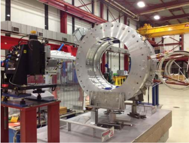
Fig. 3. TS prototype on the vibrating stretched-wire station.
