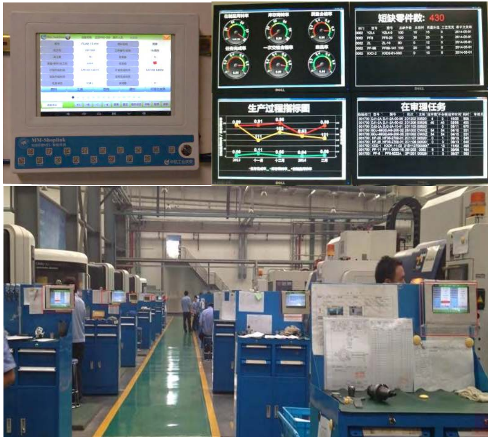
FIGURE 22. The Kanban system in the shop floor.
