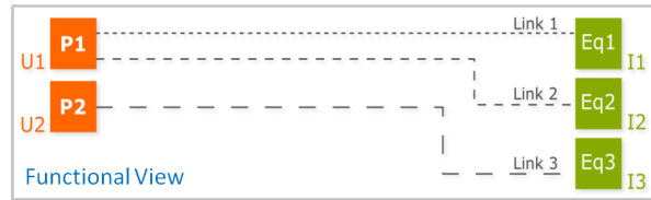
Fig. 2. A harness functional view
