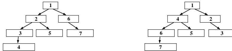
Figure 11. In the distributed deployment algorithm of Table VI, explorer agents search the partition tree \mathcal{T}_{\mathcal{P}} depth-first for leader or proxy tasks they could perform. An agent in a cell, say c_{\xi} , can always order the gap edges of c_{\xi} , e.g., counterclockwise from the parent gap edge. The depth-first search progresses by the explorer agent always moving to the next unvisited child or unexplored gap edge in that ordering. The agent thus moves from cell to cell deeper and deeper until a leaf (a vertex with no children) is found. Once at a leaf, the agent backtracks to the most recent vertex with unvisited child or unexplored gap edges and the process continues. As an example, (left) shows the depth-first order an agent would visit the vertices of \mathcal{T}_{\mathcal{P}} in Fig. 3f if the gap edges in each cell were ordered counterclockwise from the parent gap edge. If the agent instead uses a gap edge ordering cyclically shifted by one, then (right) shows the different resulting depth-first order. If each agent uses a different gap edge ordering, e.g., cyclically shifted by their UID, then different branches of \mathcal{T}_{\mathcal{P}} are explored in parallel and the deployment tends to cover the environment more quickly. Cf. Fig. 10.
