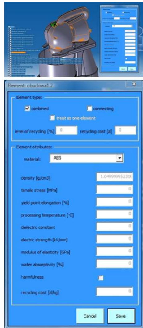
Fig. 10 Edition of combined element properties at any stage of the design process (Dostatni et al. 2014)
