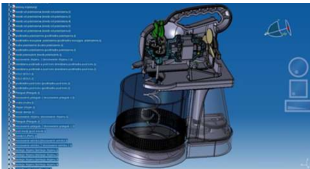
Fig. 9 Hand mixer—3D assembly model with a active view of product parts (Dostatni et al. 2014)
