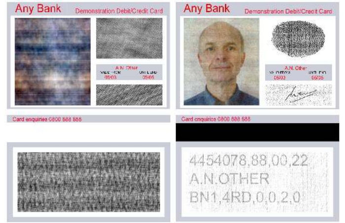
Fig. 7. Example of the application of ‘diffusion only’ watermarking. In this example, four images of a face, finger-print, signature and text have been diffused using the same noise field m and printed on the front (top-left) and back (bottom-left) of an impersonalized identity card using a 600 dpi printer. The reconstructions (top-right and bottom-right, respectively) are obtained using a conventional flat-bed scanner based on a 300 dpi grey-level scan.
