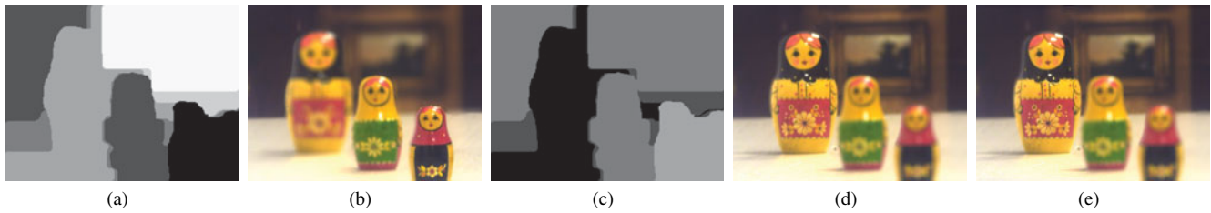
Figure 10: Refocusing on near and far objects. (a) is the computed defocus gradient map. Dark values denote small defocus gradients (i.e., points closer to the in-focus plane). Using (a) we can synthesize (b) the near focus image. (c) Defocus gradient map shifted to bring the far object to focus. (d) Synthesized refocus image using (c). (e) Synthesized refocus image using our guided deconvolution method. Notice the far object is still somewhat blurry in (d), and the detail is increased in (e).
