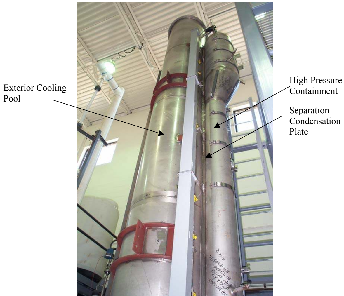
Figure 8-11 Containment and Exterior Pool Vessels of the MASLWR Test Facility
