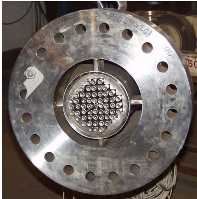
Figure 8-4 Electrically Heated Core Bundle in OSU MASLWR
