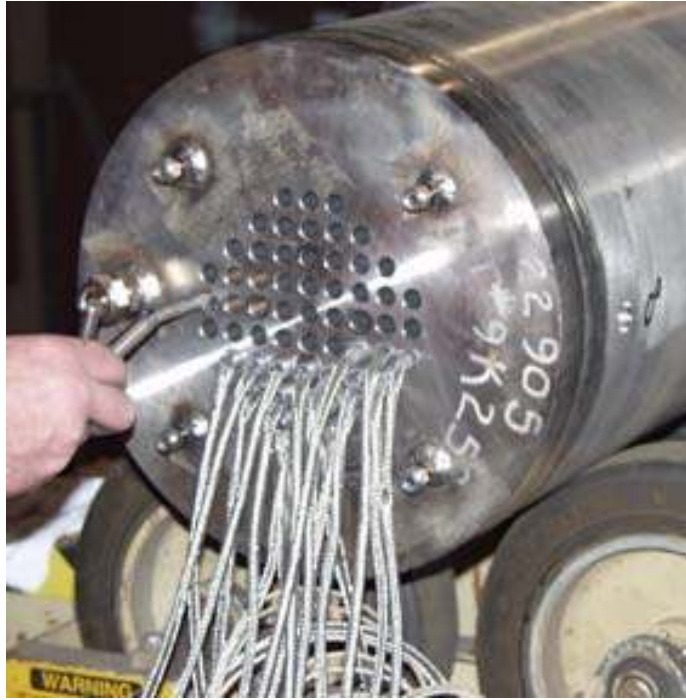
Figure 8-5 Electrical Connections for the OSU MASLWR Core Bundle (RPV Bottom Plate).
