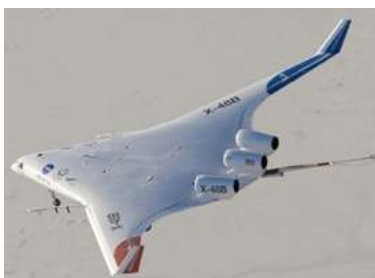
Figure 1. The Boeing X-48B Blended Wing Body, shown in flight near the NASA Dryden Flight Research Center, Edwards, California.
