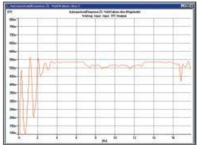
Figure 7. First order function extracted without decoupling and single pole Vold-Kalman filter.
