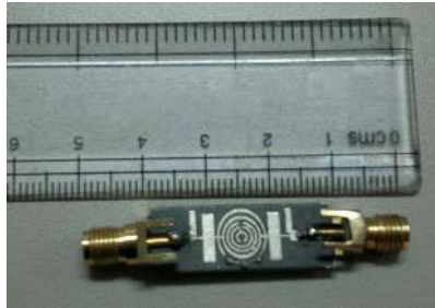
Figure 12. Fabricated UWB BPF prototype with dimensions as: W_1 = 1.8\ \text{mm} , W_2 = 0.8\ \text{mm} , W_3 = 0.4\ \text{mm} , d_1 = 1.5\ \text{mm} , d_2 = 1.5\ \text{mm} , d_3 = 0.4\ \text{mm} , L_2 = 3.9\ \text{mm} , L_3 = 7.2\ \text{mm} , A_1 = 4.4\ \text{mm} , B_1 = 3.8\ \text{mm} , A_1^* = 3.9\ \text{mm} , B_1^* = 3.5\ \text{mm} , A_2 = 3.3\ \text{mm} , B_2 = 3.0\ \text{mm} , A_2^* = 2.8\ \text{mm} , B_2^* = 2.8\ \text{mm} , g_1 = 0.6\ \text{mm} , g_2 = 0.5\ \text{mm} , g_3 = 0.4\ \text{mm} , g_4 = 0.5 , g_5 = 1.0\ \text{mm} , g_6 = 0.7\ \text{mm} , R_1 = 2.4\ \text{mm} , R_2 = 1.9\ \text{mm} , R_3 = 0.9\ \text{mm} , W_4 = 0.22\ \text{mm} , W_5 = 0.25\ \text{mm} , P_1 = 0.3\ \text{mm} , S_1 = 0.1\ \text{mm} and P = 0.4\ \text{mm} .
