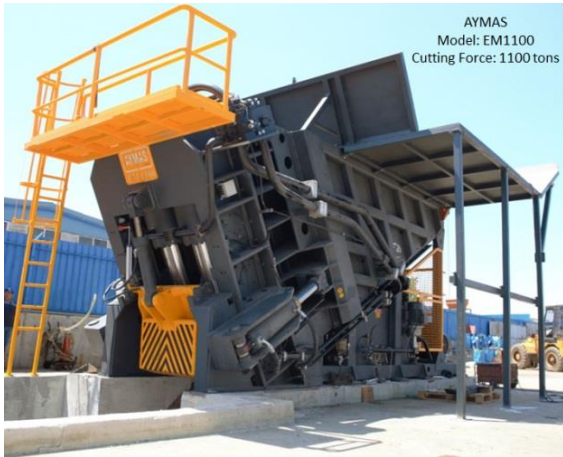
Fig. 1 Inclined scrap shear
