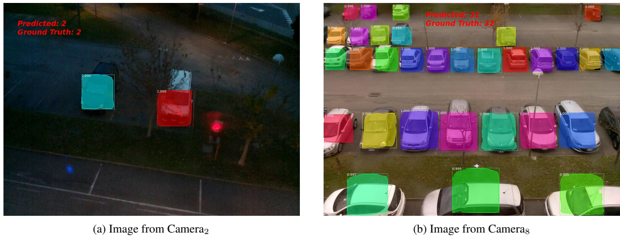
Figure 4: Two examples of the output of our counting method. Images are taken from the CNRPark-EXT dataset. We report the predictions and the estimate of the number of vehicles present in the scene.
