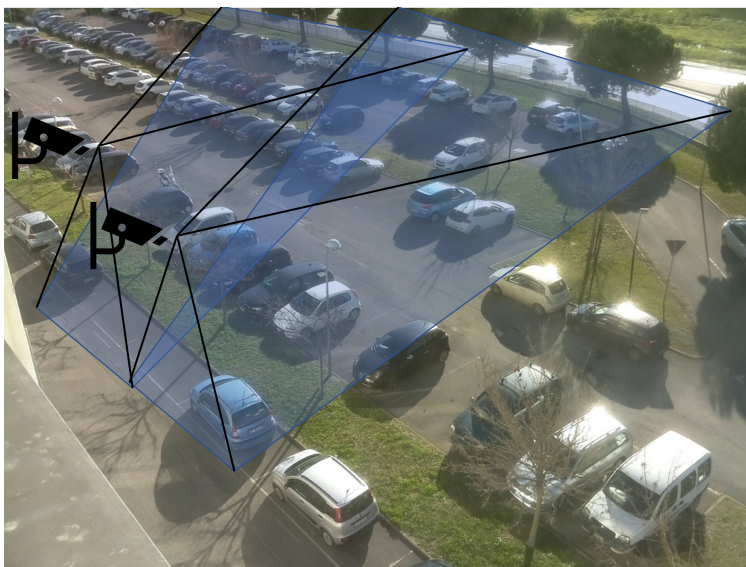
Figure 1: An example of two cameras monitoring the same parking area with partially overlapping fields of views. This redundancy provides robustness and fault-tolerance but also raises the problem of aggregating knowledge extracted from the individual cameras.
