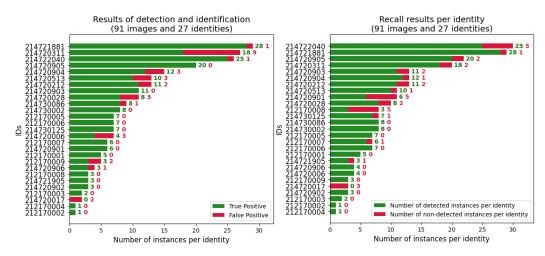
**Figure 9.** Precision and recall results. (**Left**) The precision of the detection and identification per identity with the mean precision achieving 88.14%. (**Right**) The recall of detection and identification per identity with a mean value of 86.43%. Best viewed in color.
