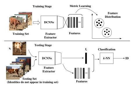
**Figure 1.** Pipeline of the cattle identification model training and testing under the open-set identification protocol. In the training stage, the deep metric learning methodology is utilized to supervise the learning process to extract separable and discriminative features. In the testing stage, the feature is extracted using DCNNs and classified by the *k*-NN classifier.
