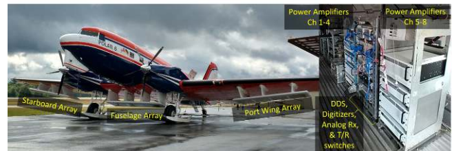
Figure 3: Photographs of the BT-67 aircraft (Polar 6) equipped with 3 antenna sub-arrays and skis (left); and the radar electronics installed inside the cabin (right).
