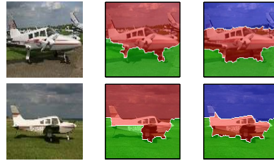
Figure 2. This figure shows how increasing the number of classes leads to a better segmentation. Columns 2 to 3 respectively show results for K = 2 and K = 3 (best seen in color).
