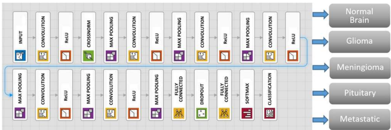
Fig. 3 Architecture of the proposed CNN model for Classification-2 task
