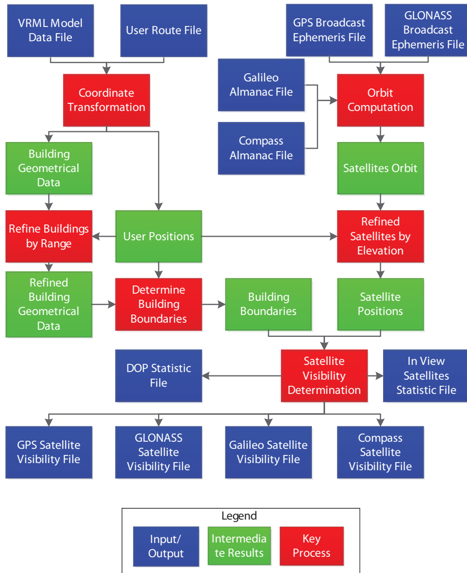
Figure 2. Software flowchart for satellite visibility determination.
