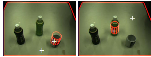
Cup detection result using 3D feature points (left : success, right : fail)
