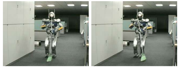
Fig. 4. Tool manipulation behaviors of a humanoid Both sweeping and vacuuming behavior are able to generate using object models, tool manipulation knowledge and trajectories of a manipulation coordinate.
