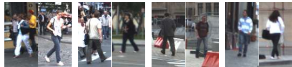
Figure 8: Sample detections for the different models learned by MPLBoost (K=4) using HOG, Haar, IMHwd. The models to the left respond more strongly to side/45-degree views, the models to the right to front/back views.
