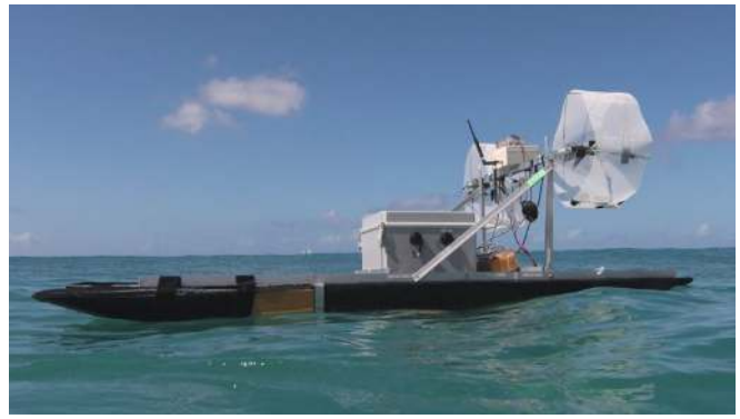
Fig. 5. The Marine Autonomous Robotic Explorer (MARE) is a catamaran robotic airboat that can operate in turbulent open water environments.
