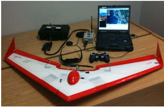
Fig. 4. The Unicorn is a fixed-wing UAV with an on-board autopilot microprocessor and a gimbal-mounted camera.
