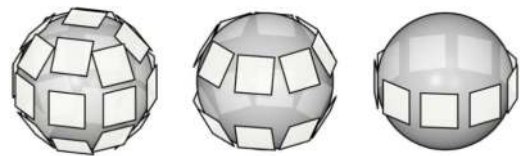
FIGURE 3. Uniform (left), tropical (center), and equatorial (right) viewports sampling for computing viewport-based objective metrics.
