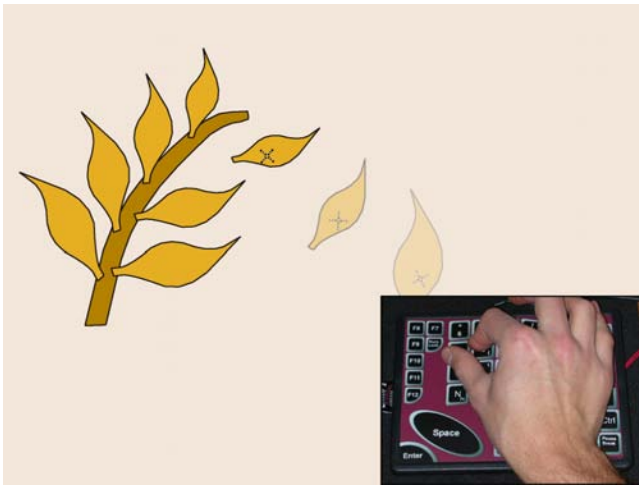
Figure 3: A user simultaneously translates, rotates, and scales a leaf using the Similarity Cursor. Parallel control of an object’s properties allows for more fluid interaction, and may decrease task completion time.
