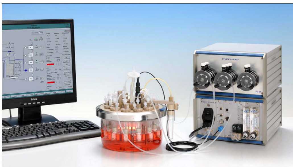
Fig. (1). The Multiferm multi-fixed-bed fermenter system. Middle: Conditioning vessel with the 12 single fixed-bed units. Left: Process control system WinErs. Right: Control unit for feed, harvest, pH, aeration and temperature (medorex e.k., with kind permission).
