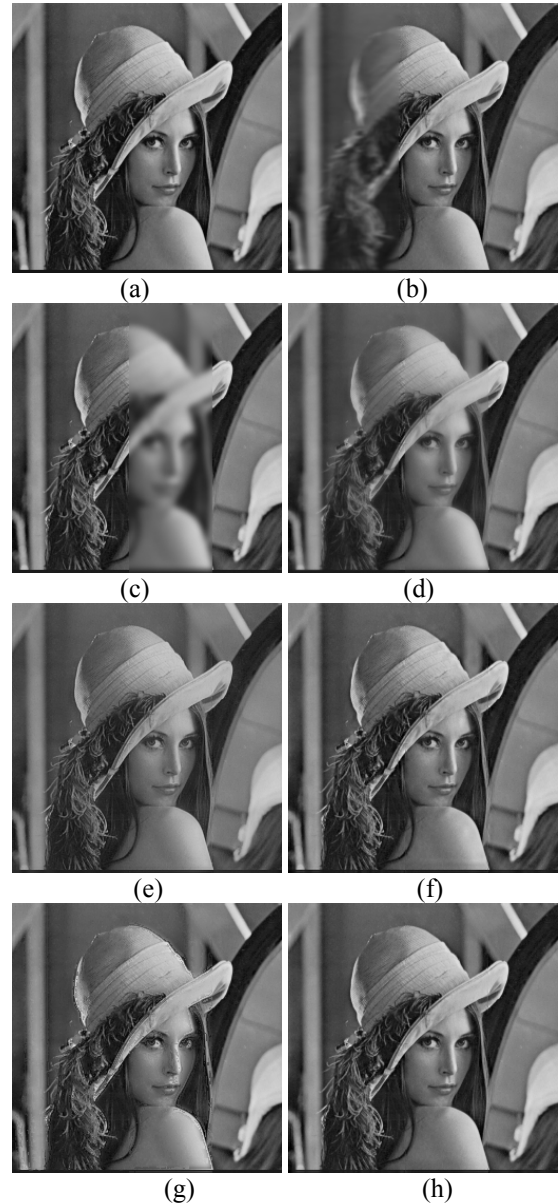
Fig.1. Image fusion with the simulated pair from Lena image. (a) The original image (reference image or ground truth); (b) image blurred on the left; (c) image blurred on the right; (d) fused image by pixel averaging; (e) fused image by FSD pyramid; (f) fused image by DWT; (g) fused image by the method of [21]; (h) fused image by the proposed method.
