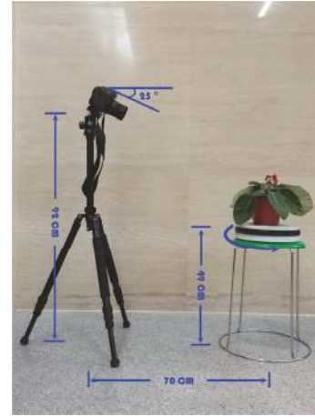
FIGURE 2: Image acquisition and equipment setup.
