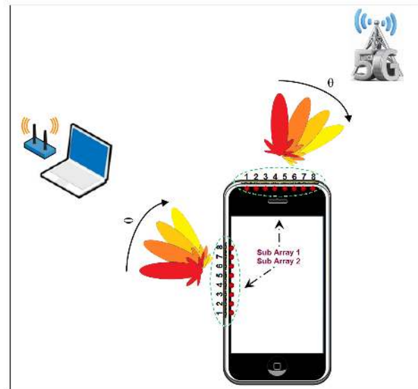
Fig. 2. Architecture of the multi-user MIMO for 5G mobile communications.
