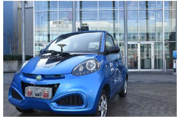
Fig. 1. Picture of the testing car. Perception sensors are visible on the roof (Velodyne and cameras) and on the front bumper ( radars and laser).
