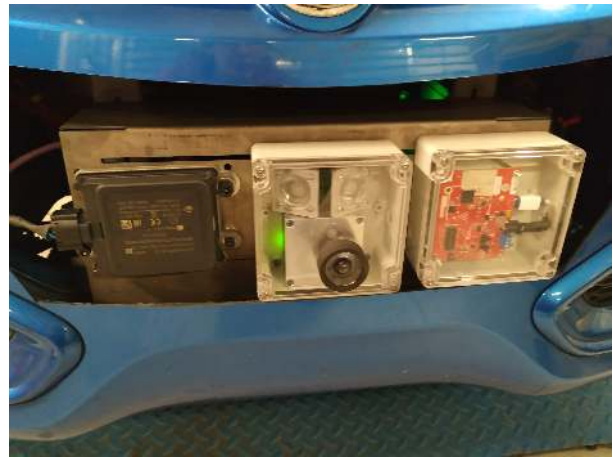
Fig. 3. Detail of the sensors mounted on the front bumper, from the left to the right, Continental radar, Leddartech M16 solid state laser and Texas instrument radar
