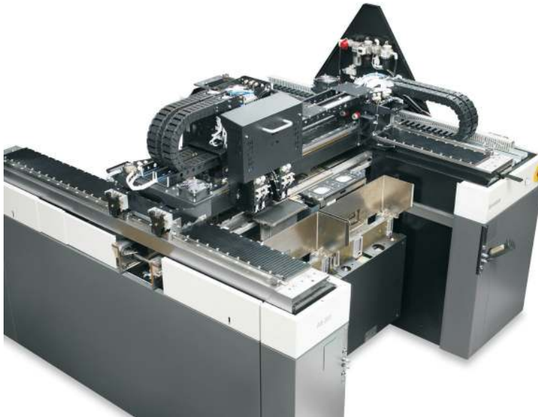
Figure 1.2: Interior of an Assembléon AX201 surface mount machine
