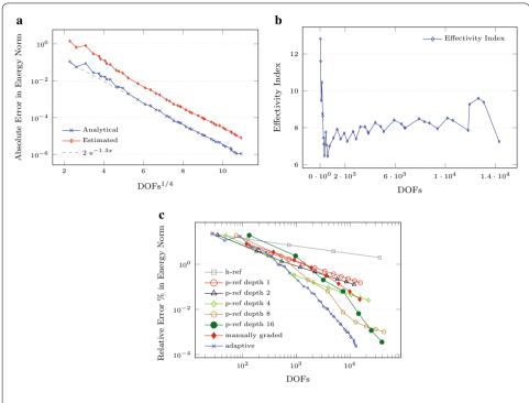
Fig. 8 Singular cube: error estimates, effectivity index and convergence. **a** Error estimates and convergence rate. **b** Effectivity index. **c** Convergence comparison
