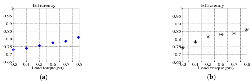
Figure 11. Total efficiency of the system: (a) 3LI PWM operated; (b) 3LI+TLI5 configuration.
