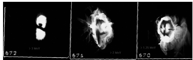
Figure 4: Images of the emitted proton beam at different energies using CR-39. Image 672, above 3 MeV; 671 above 3 MeV; and 670 above 1.35 MeV
