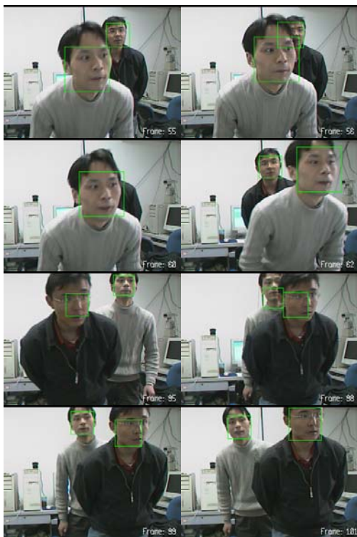
Figure 8. Tracking of multiple faces: occlusions handling. (Frame 55,56,60,62 and 95,98,99,101)
