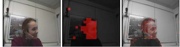
Fig. 2. Compressed-domain video features: From left, original, detected skin-color blocks, motion vectors.
