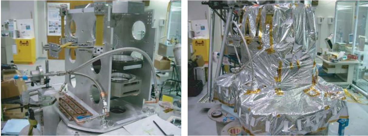
Fig. 7. Precooling system (left) and optical-bench plate covered by MLIs (right). (Copyright SPIE [2006].)
