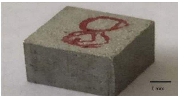
Fig. 3 Specimen prepared after machining
